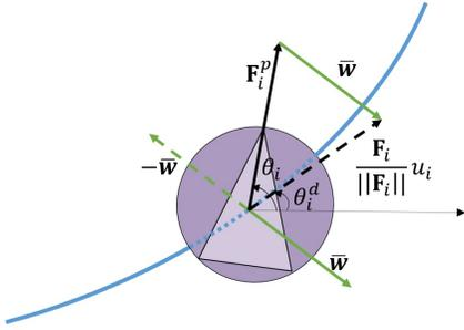
Fig. 2. Construction of new vector field in the presence of wind. Blue line is the desired trajectory, green arrow, dotted black arrow and solid black arrow show the direction of the mean wind speed, nominal vector field  $\mathbf{F}_i$  and constructed vector field  $\mathbf{F}_i^p$  respectively.
