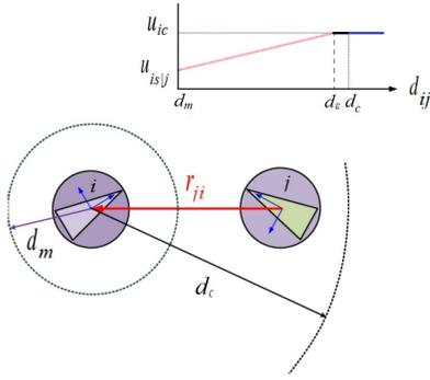
Fig. 1. If  $J_j \triangleq \mathbf{r}_{ji}^T \boldsymbol{\eta}_i < 0$ , i.e., if agent  $i$  moves towards agent  $j$ , then agent  $i$  adjusts its linear velocity according to the velocity profile shown here, given analytically by (8).
