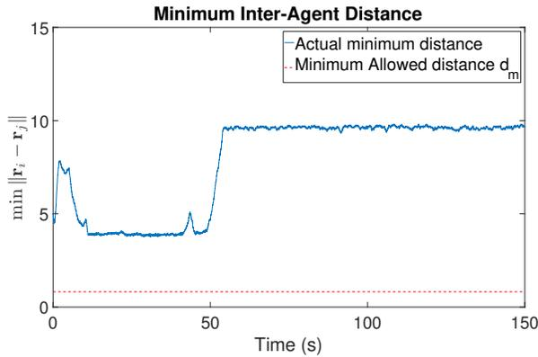
Fig. 5. Smallest pairwise distance for time varying  $\bar{w}$ .
